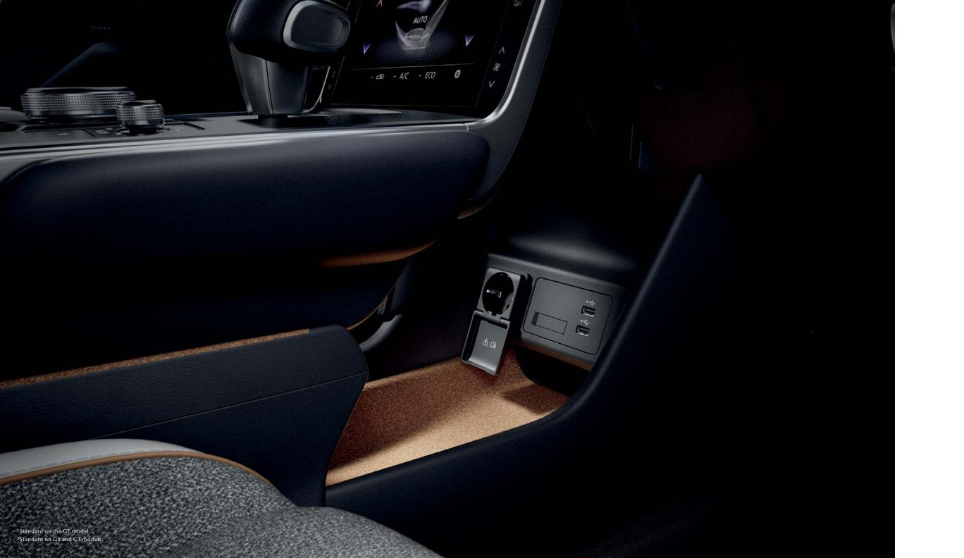
**Left:** 120 V 150 W AC power outlet<sup>1</sup> and dual USB ports,<sup>2</sup> under the floating centre console.
